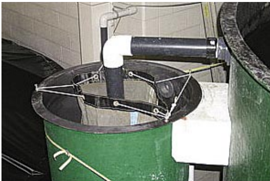
Figure 2. Egg collection utilising an external collection tank. The bag is connected to the overflow pipe of the broodstock tank (Photo courtesy of The Ocean Sciences Centre, Newfoundland).
