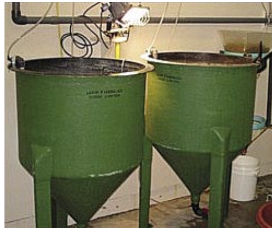
Figure 6. Artemia production tanks. A "decapsulation cone" can be seen at the far right. Dehydrated cysts, purchased from a supplier, have to be decapsulated before the hatching process can begin. Artemia grow and receive enrichment in these tanks before being transferred to the larval tanks. (Photo courtesy of The Ocean Sciences Centre, Newfoundland).
